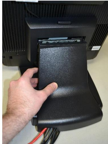
37. Locate the button cover panel on the left-hand side of the touchscreen. Press in the center of the panel to open.
