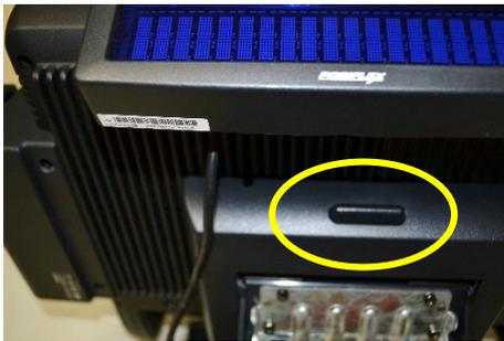
17. Position one hand underneath the touchscreen. Press the release button with your other hand.
