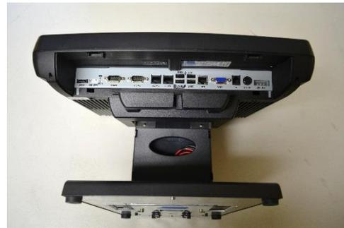
14. Locate the 'COM1' port to the left of the accessory ports.
