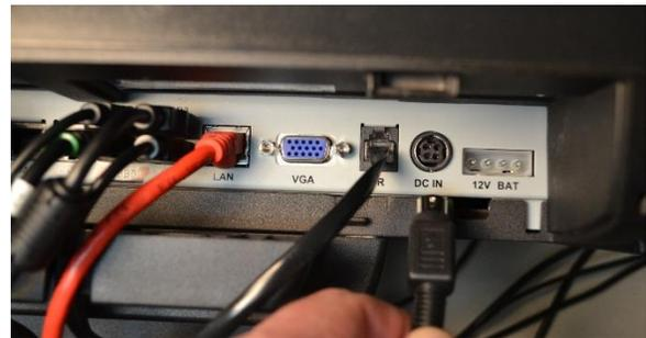
32. Connect the battery back-up to the '12V BAT' port.
