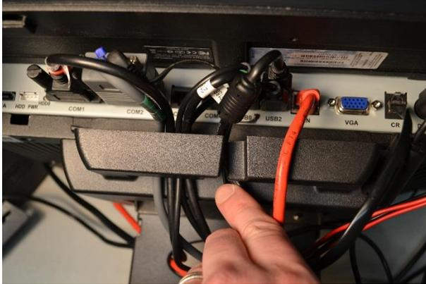
34. Slide the cable cover back into place. Swivel the touchscreen back into an upright position.
