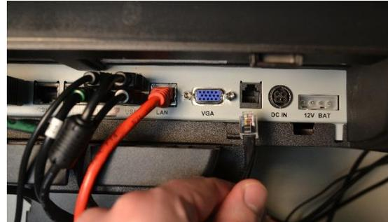
31. Connect the touchscreen's power supply cable to the 'DC IN' port
