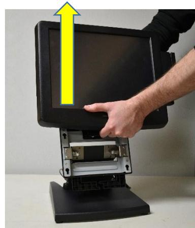
19. Note the touchscreen is connected to the base unit by four pins that key into corresponding slots on the base unit.
