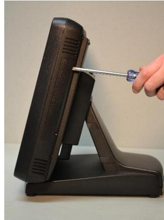
3. Remove the panel. The connector for the card reader will be visible.
