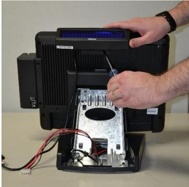
16. Locate the touchscreen release button on the top rear of of the base.
