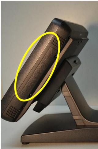
2. Remove the two screws that attach the panel to the touchscreen.
