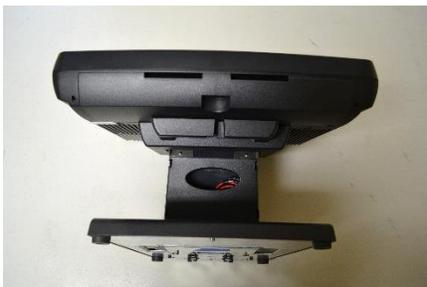
12. Locate the two locking tabs for the port cover. Gently press down on these tabs and slide the cover away from the touchscreen.
