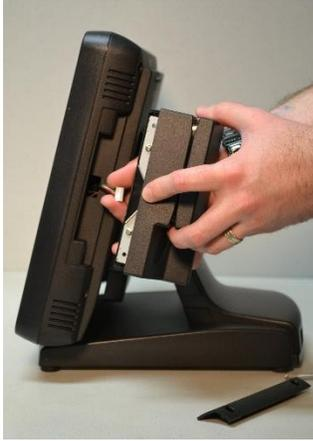
6. Attach the card reader to the touchscreen with the same two screws previously removed.
