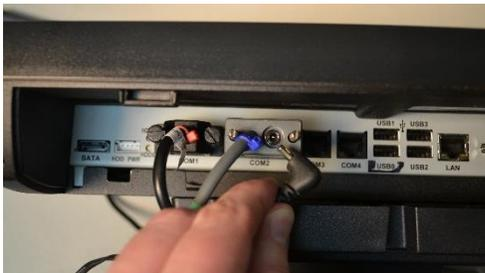
28. Connect all USB devices, such as a keyboard, mouse, signature capture device, etc. to the USB ports.
