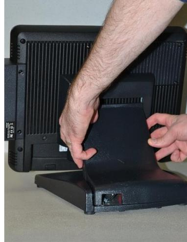
8. Remove the cover by gently prying up on the four tabs holding it in place and lift away.
