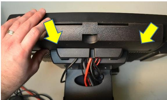
35. At the rear of the touchscreen, gather all of the cables into the lower-left-hand corner of the base (except the customer display cable).
