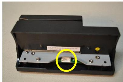
5. Insert the connector from the touchscreen into the port on the card reader.
