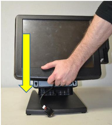
23. Make sure the customer display cable is properly routed through the notch and all four pins are properly seated in their corresponding slots on the base unit.
