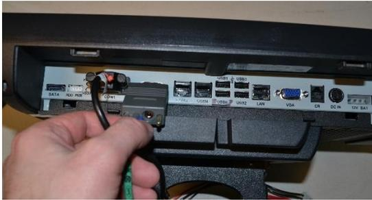
27. Insert the power supply plug into the hand scanner plug.
