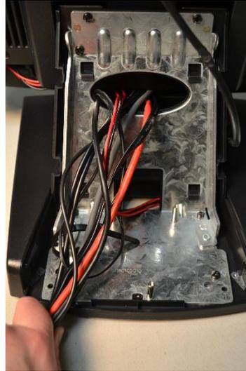
36. Press the cable cover back into place making sure the customer display cable remains clear if equipped. Power on all peripheral devices at this time.
