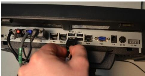
29. Insert the network cable into the 'LAN' port.
