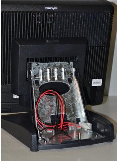
10. Swivel the touchscreen back to access the port cover at the bottom of the screen.
