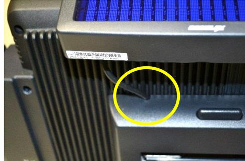
24. Connect the customer display cable to the 'COM1' port.
