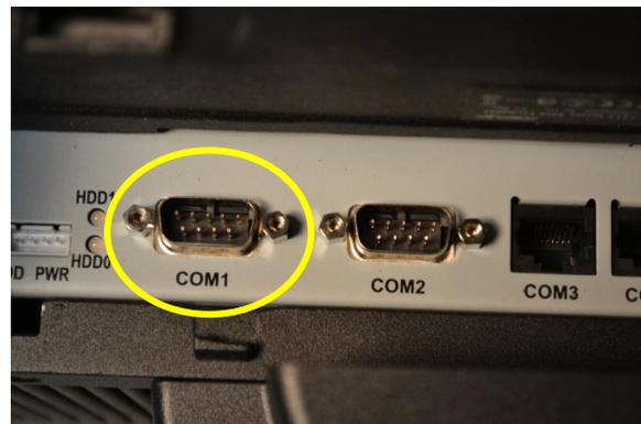
NOTE: 'COM1' *must* either have an accessory or the COM terminator connected plugged into it.
