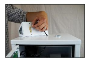
Align SecurVision camera over drill hole and ensure camera face is parallel to front of chassis.
