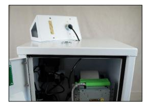
8. Apply generous amount of silicon to perimeter of SecurVision camera to ensure tight waterproof seal.
