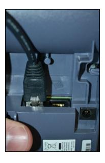
4. Route AC adaptor cable through cable keeper notch and connect it to power port.
