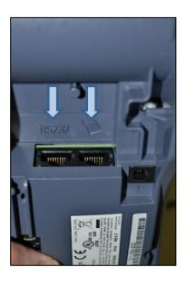
2. Connect the RS232 end of the Pioneer cable to the RS232 port.
