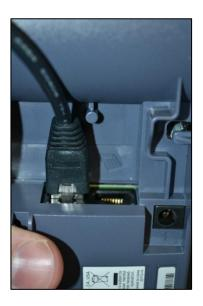
3. If using an optional external keypad (not supplied), connect it to keypad port.
