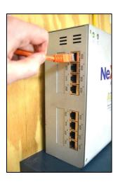
4. Connect Cat6 Ethernet cable (not supplied) to RJ-45 network port.
