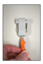
2. Connect serial adaptor to serial port.
