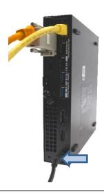
7. Connect VGA cable (not supplied) to VGA display adaptor.
