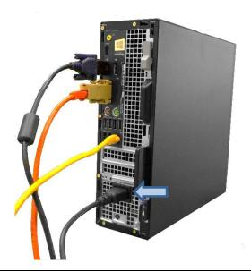
2. Connect Ethernet cable to Ethernet port, then connect other end of cable to network switch (not supplied).
