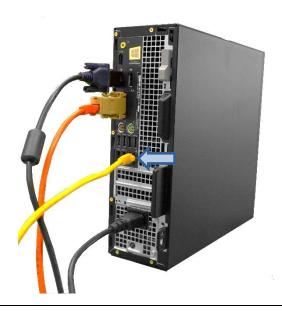
3. Connect Cat6 cable to 9-pin serial adaptor.
