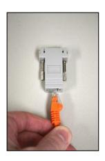
4. Connect serial adaptor to serial port, then connect other end of Cat6 cable to fuel controller (port number varies depending on your dispenser brand).
