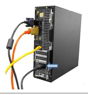
3. Connect Cat6 cable to 9-pin serial adaptor.
