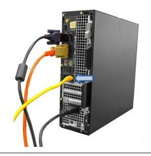
4. Connect serial adaptor to serial port, then connect other end of Cat6 cable to fuel controller (port number varies depending on your dispenser brand).
